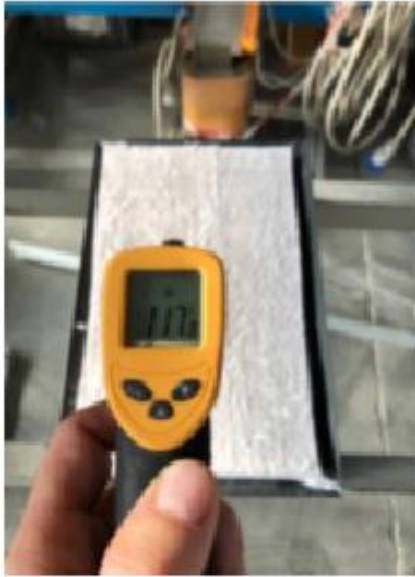
Picture 8: Other material end test – rear temperature 320 °C
